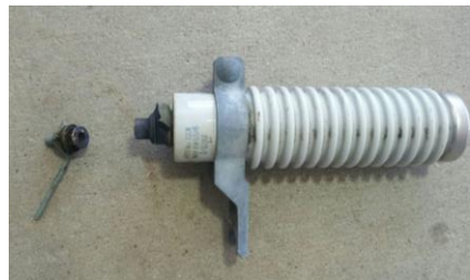
DFA technology enabled detection and identification of a failed arrester, thereby improving response.
