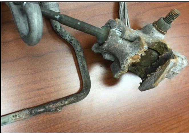
Fig. 15. Hotline clamp and stirrup found after one week of series arcing
