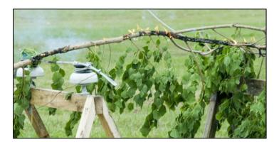
then transition suddenly to a high-current flashover. The prolonged, low-amplitude flow of current can damage the conductor, at the points of contact, as can any high-amplitude flashover events that may occur. The aforementioned process occurs when the branch contains moisture. Almost no measurable current flows when the branch is dead and well dried [1,2].
