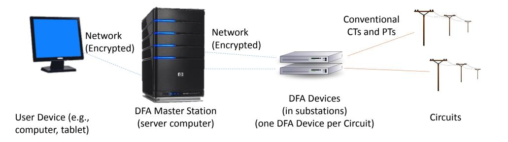
Each substation-installed DFA Device runs waveform analysis and classification software and then sends results to a central DFA Master Station. Personnel access DFA results via browser connection to the DFA Master Station.
